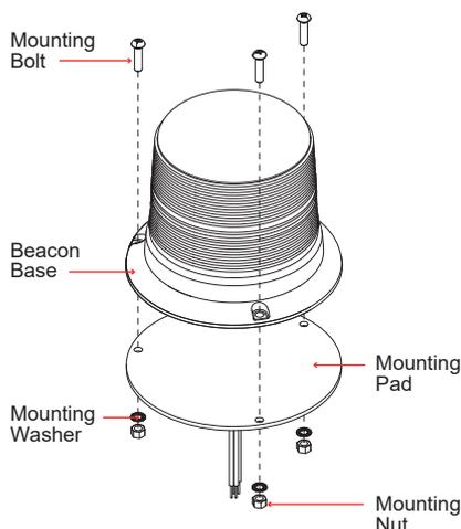
1. Drill holes on the mounting surface for the wire-exit and mounting bolts.
